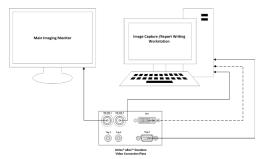
Connection of a Digital Video Recorder using the HD-SDI 2 or the DVI Video Signal and TRIG 1 and/or TRIG 2
