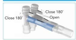
Operation of the Y-connector available with the VivaSight 2 DLT. In the illustration, both lumens are open for ventilation.
